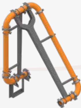
Pipeline Scissors (slip-form pipeline connection)
