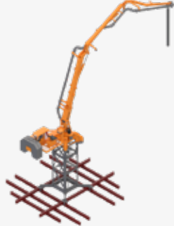
Short-Outriggers with Ballast Weights (Freestanding)
